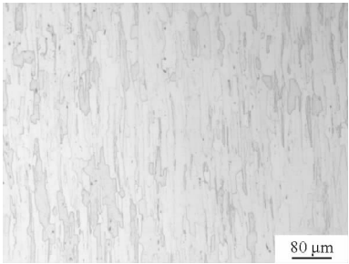
图 2 固溶态 7050 铝合金板材横截面显微组织 Fig.2 Cross-section microstructure of solid-soluted 7050 plate
